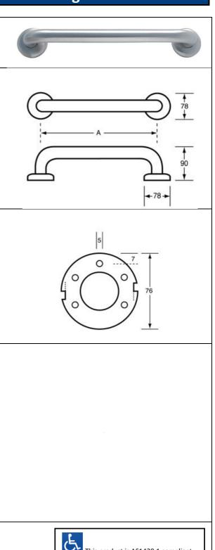
This product is AS1428.1 compliant (accessible compliant) when installed in accordance with the guidelines.
